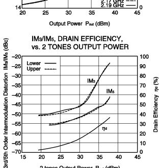
W-CDMA 3GPP, Test Model 1,• 64 DPCH, 67% Clipping, Center Frequency 2.14GHz, 15 MHz spacing
