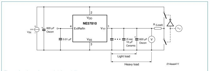
Fig 14. Load transient test (+3 A to -3 A)
