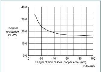
Fig 7. PCB heat sink area versus thermal resistance
