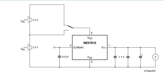
Fig 16.  $V_{DD}$  to  $V_{TT}$  transient test
