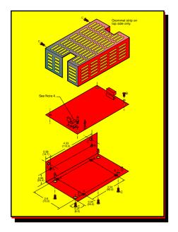
Bracket outside dim. 5.49" x 3.43" x 1.88" (139.5 x 87.2 x 47.9mm) Cover outside dim. 5.49" x 3.38" x 1.82" (139.5 x 85.8 x 46.3mm)
