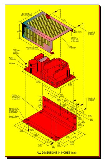
Bracket outside dim: 7.3" x 4.45" x 2.6" (185.42 x 113.03 x 66.04mm) Cover outside dim: 6.5" x 4.45" x 2.54" (165.10 x 113.03 x 64.52mm)
