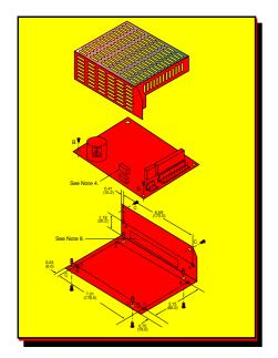
Bracket outside dim: 7.5" x 4.57" x 2.38" (190.5 x 116 x 60.5mm) Cover outside dim: 7.5" x 4.51" x 2.32" (190.5 x 114.5 x 59mm)
