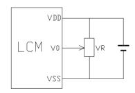
VDD~V0: LCD Driving voltage
