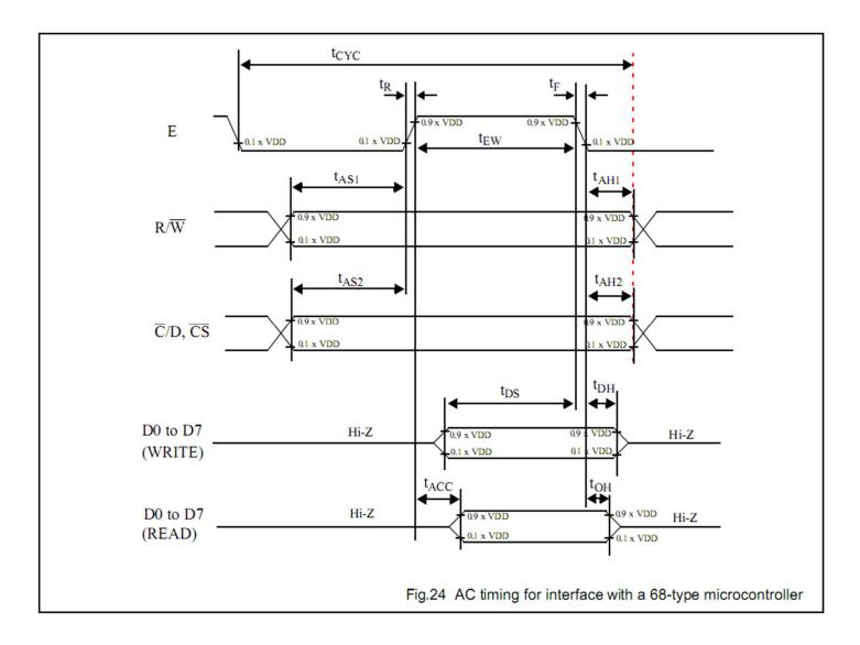
$V_{DD}$  = 5 V ±10%;  $V_{SS}$  = 0 V;  $T_{amb}$  = -20 °C to +75°C.
