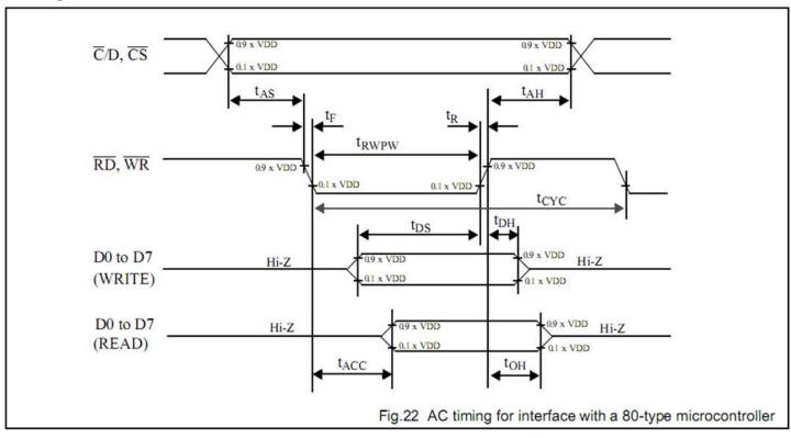
$V_{DD}$  = 5 V ±10%;  $V_{SS}$  = 0 V;  $T_{amb}$  = -20 °C to +75°C.
