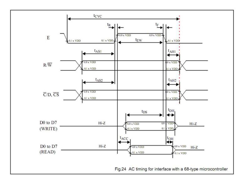
$V_{DD}$  = 5 V ±10%;  $V_{SS}$  = 0 V;  $T_{amb}$  = -20 °C to +75°C.
