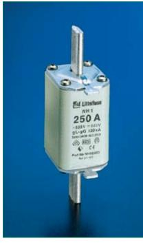
Littelfuse European style NH fuse links are designed for the protection of conductors and motors. The gL-gG characteristic fuse links are generally used to protect cables and installation lines from overloads and short-circuits. The aM characteristic fuse links are used for the short-circuit protection of motors and switchgear. They are available in NH00C to NH3 sizes up to 630 amperes.
