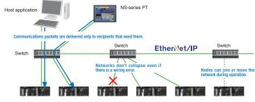
Star topology using Ethernet switch technology
