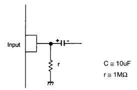
This IC requires  $0.1\mu$ F capacitor between INPUT and GND,  $1M\Omega$  resistance between INPUT and GND for clamp type input at mute mode.
