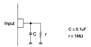
This IC requires  $0.1\mu$ F capacitor between INPUT and GND for bias type input at mute mode.
