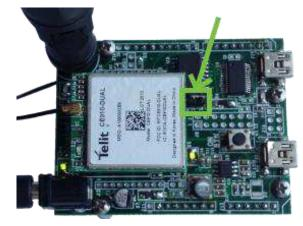
2.4 Plug in 12V Power Supply to connector J15
