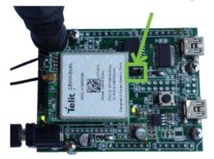
3.4 Plug in 12V Power Supply to connector J15
