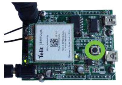
Note: LEDs D1 on baseboard and D1 on module flash ON momentarily.
