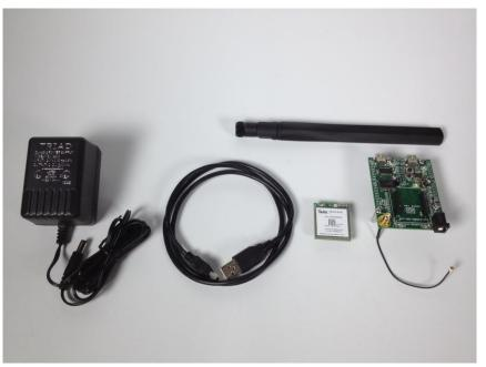
Note: Photo depicts modem removed from baseboard, however, modem ships pre-mounted to baseboard for ease of assembly.
