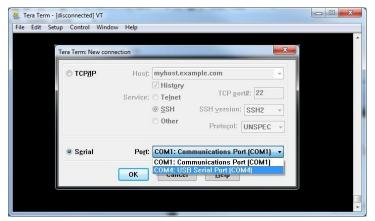
Serial Settings should be as follows: Baud Rate: 115,200 bps Data: 8bit Parity: none Stop: 1bit Flow Control:none
