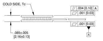
CERAMIC MATERIAL: ALUMINA (AC) MILLIMETERS ARE IN []
