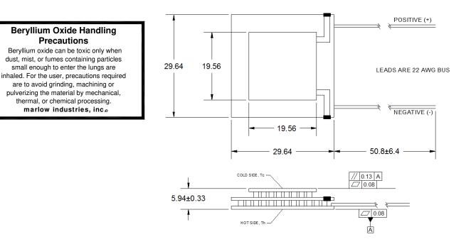
Ceramic Material: Combination of Alumina and Beryllia (AB) All units are in millimeters unless otherwise stated.
