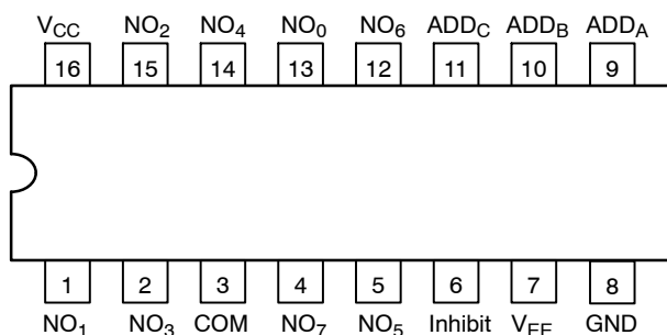
Figure 1. Pin Connection (Top View)
