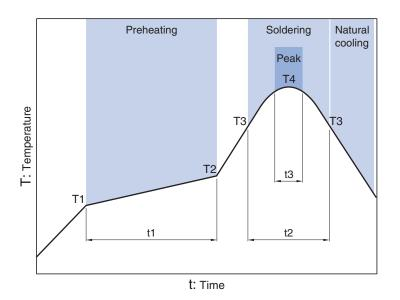
Preheating Soldering Peak Temp. Time Temp. Time Temp. Time T1 T2 t1 тз t2 Т4 t3 150°C 180°C 90 to 120s 230°C 255°C 40s 10s max.
