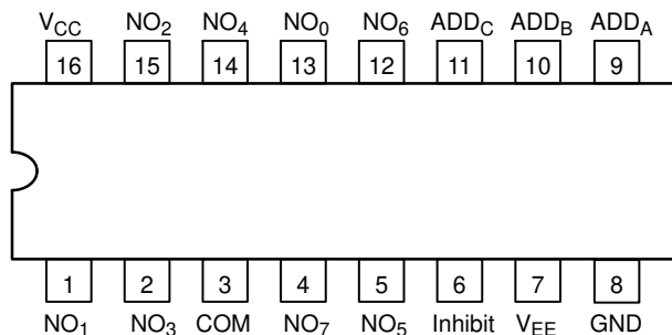
Figure 1. Pin Connection (Top View)
