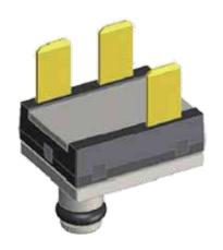
NovaSensor's NPR-101 pressure sensor is a silicon-based MEMS device using "Backside Absolute Pressure" technology designed for harsh media exposure, which eliminates the direct contact of the sensing circuitry with the applied media. The device is coupled with an ASIC to provide a ratiometric output proportional to the applied pressure. Integrated diagnostics included.
