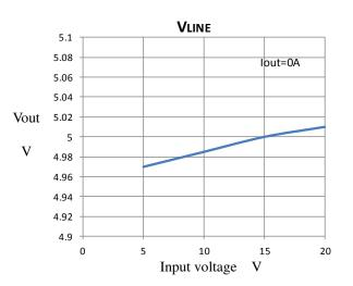
(2)Input voltage vs. Output
