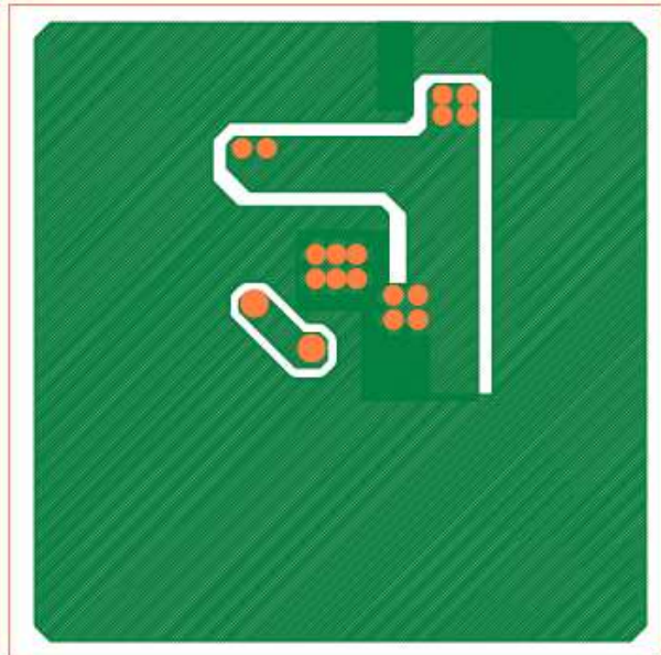
Back Side: GND Side (double sided board)
