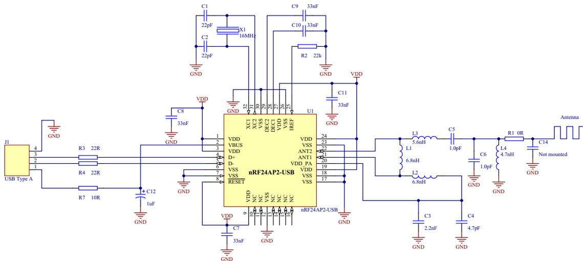
Figure 1. nRF24AP2-USB schematic
