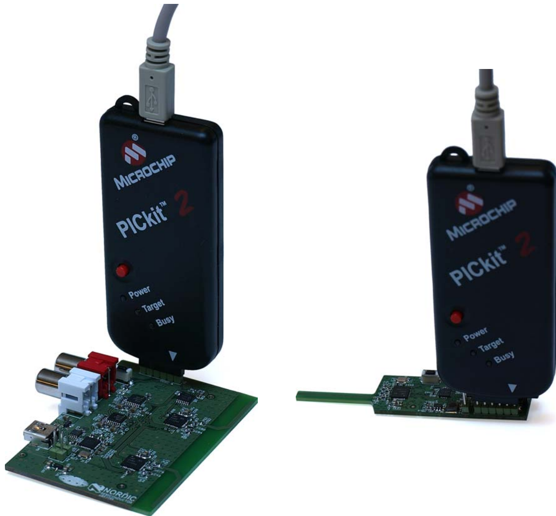
Figure 3. Receiver board and microphone setup with PICkit2™
