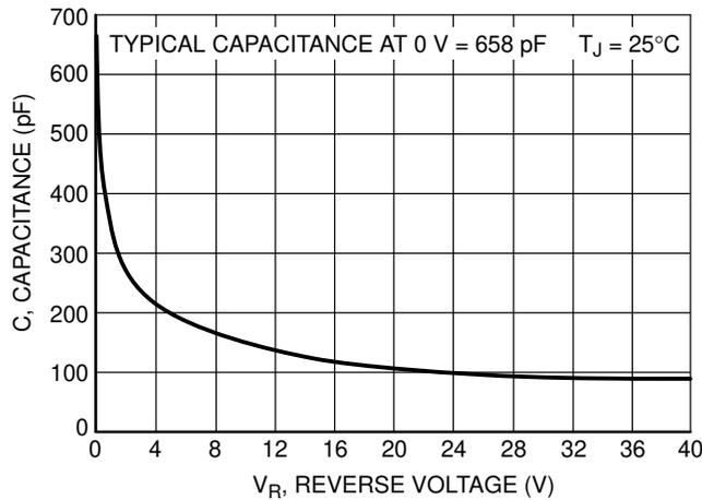
**Figure 7. Typical Capacitance**
