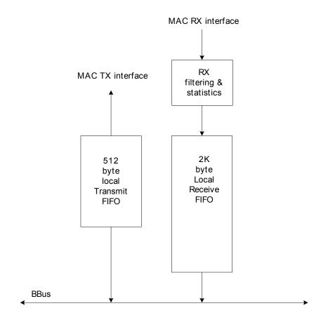
Figure 4: EFE module block diagram
