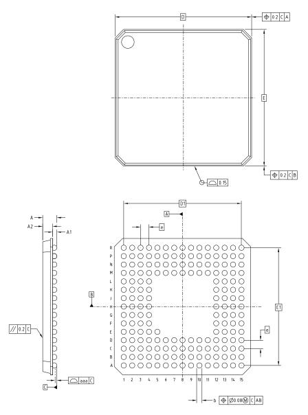
Figure 2: NS7520 pinout and dimensions
