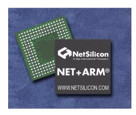
The NS7520 can support most any networking scenario, and includes a 10/100 BaseT Ethernet MAC and two independent serial ports (each of which can run in UART or SPI mode).
