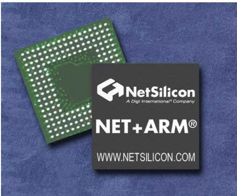
The NS7520 can support most any networking scenario, and includes a 10/100 BaseT Ethernet MAC and two independent serial ports (each of which can run in UART or SPI mode).
