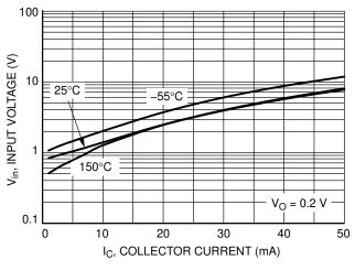
Figure 11. Input Voltage vs. Output Current
