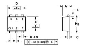
NOTES: 1. DIMENSIONING AND TOLERANCING PER ANSI Y14.5M, 1982. 2. CONTROLLING DIMENSION: MILLIMETERS 3. MAXIMUM LEAD THICKNESS INCLUDES LEAD FINISH THICKNESS. MINIMUM LEAD THICKNESS IS THE MINIMUM THICKNESS OF BASE MATERIAL.
