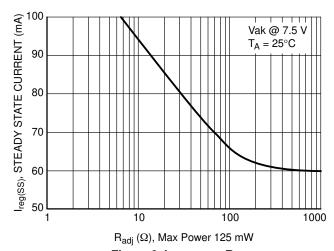
Figure 6. I<sub>reg(SS)</sub> vs. R<sub>adj</sub>
