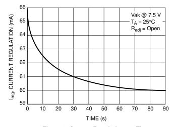
Figure 5. Current Regulation vs. Time
