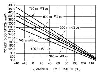
Figure 7. Power Dissipation vs. Ambient Temperature @  $T_J = 175$ °C
