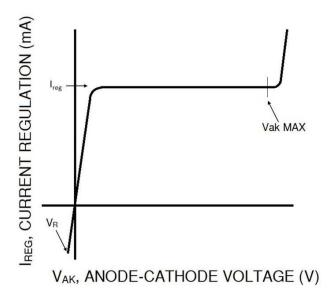
Figure 1. CCR Voltage-Current Characteristic
