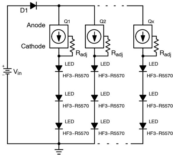
**Figure 8. Typical Application Circuit (30 mA each LED String)**
