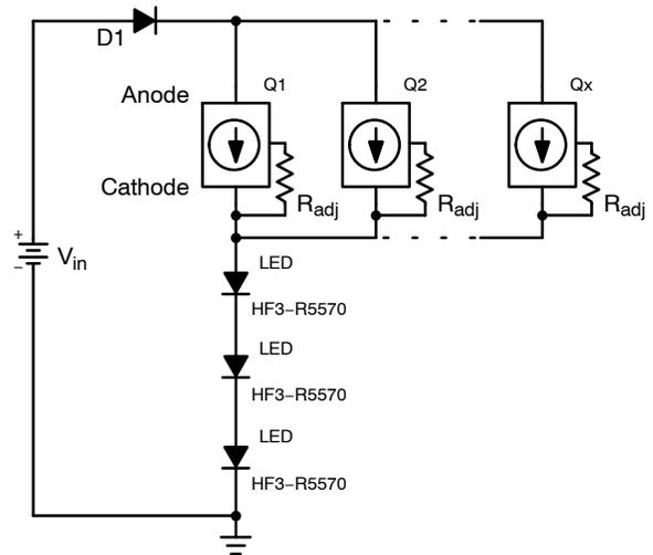
**Figure 9. Typical Application Circuit (90 mA each LED String)**
