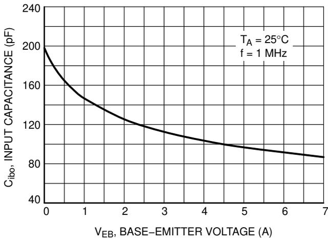
Figure 9. Input Capacitance
