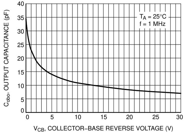
Figure 10. Output Capacitance
