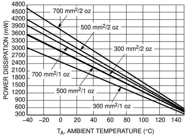
Figure 7. Power Dissipation vs. Ambient Temperature @  $T_J = 175^\circ\text{C}$
