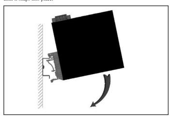
To remove the unit from the DIN rail, place a flat head screwdriver into the release clip found at the bottom of the unit, and apply downward force on the clip until it disengages the bottom of the unit from the DIN rail. Rotate the bottom of the unit towards you and up at an approximate 15° upward angle to completely remove the unit.
