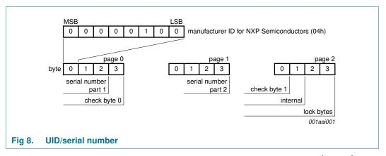
In accordance with ISO/IEC 14443-3 check byte 0 (BCC0) is defined as CT Å SN0 Å SN1 Å SN2 and check byte 1 (BCC1) is defined as SN3 Å SN4 Å SN5 Å SN6.
