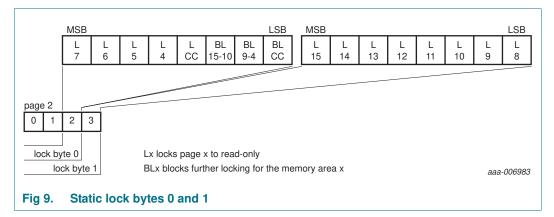
For example if BL15-10 is set to logic 1, then bits L15 to L10 (lock byte 1, bit[7:2]) can no longer be changed. The so called static locking and block-locking bits are set by a WRITE or COMPATIBILITY\_WRITE command to page 02h. Bytes 2 and 3 of the WRITE or
