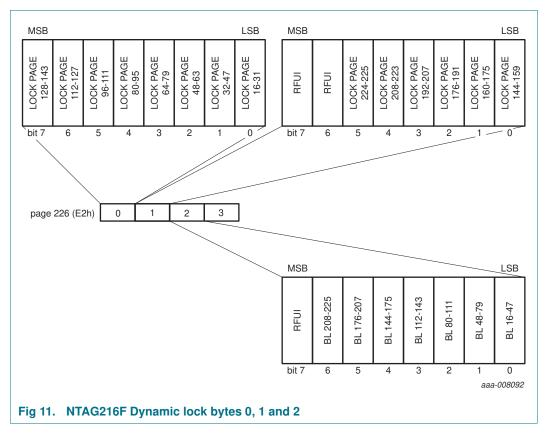
The default value of the dynamic lock bytes is 00 00 00h. The value of Byte 3 is always BDh when read.
