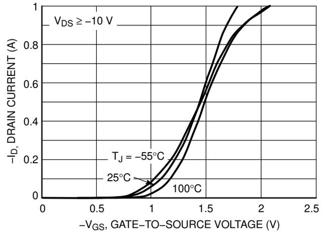
Figure 2. Transfer Characteristics
