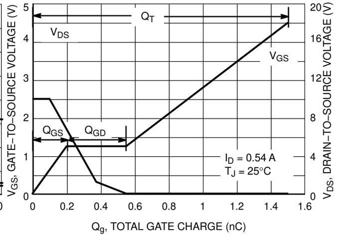
**Figure 8. Gate-to-Source and Drain-to-Source Voltage versus Total Charge**
