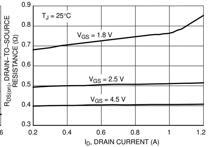
Figure 4. On-Resistance versus Drain Current and Gate Voltage
