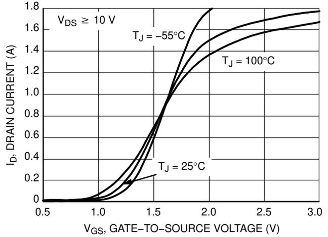
Figure 2. Transfer Characteristics
