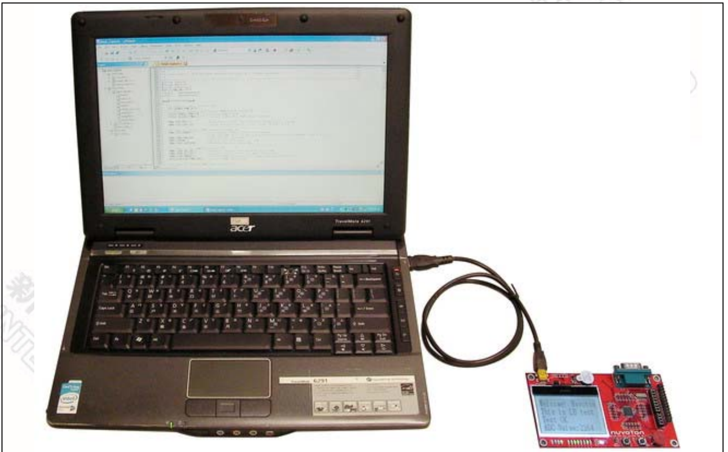
Figure 3-1 Nu-LB-M051 Hardware Setup
