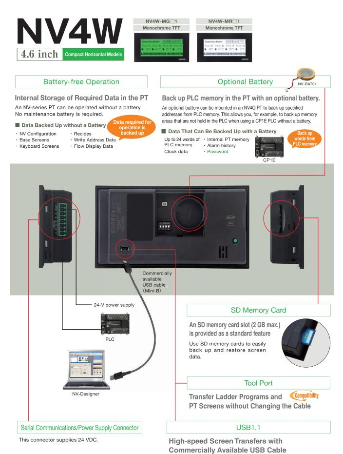
A USB interface is provided to effectively use computer software environments.Screens that are created on the computer can be quickly transferred to the PT using a commercially available USB cable (Mini-B).
