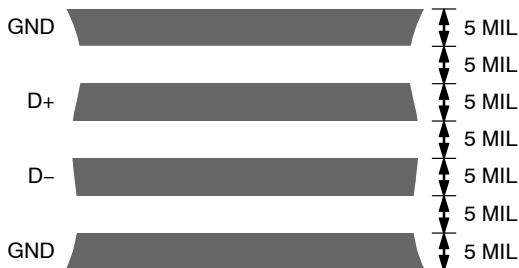
Figure 22. Typical Arrangement of Signal Tracks
