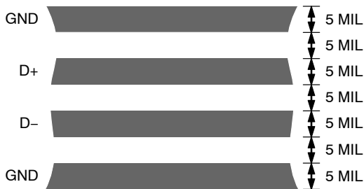
Figure 22. Typical Arrangement of Signal Tracks
