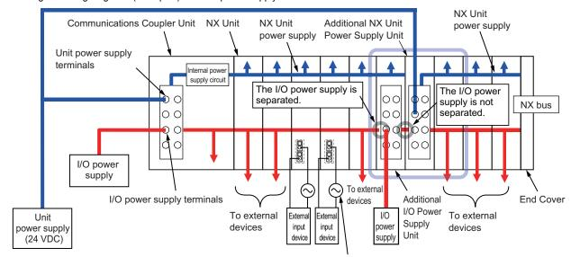
I/O power supply (Supply from external source)
