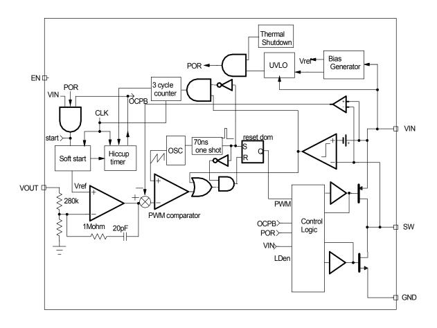
Figure 2 - Simplified block diagram of the NX4108-15
