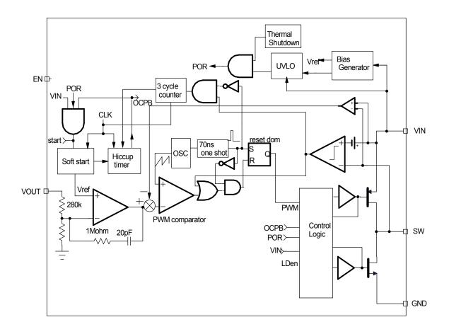
Figure 2 - Simplified block diagram of the NX4108-18
