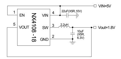
Figure 1 - Typical application of NX4108-18
