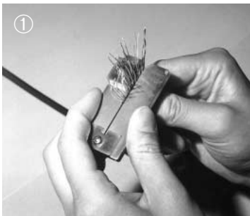
1. Set the wires in the wiring fixtures.
