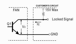
\*Transistor Q1 at "ON" position Collector current.....I<sub>c</sub>=10mA Max Saturation Voltage.....V<sub>oL</sub>=1.0V Max (Between Collector and Emitter at I<sub>c</sub>=10mA) \*Transistor Q1 at "OFF" position Release Voltage.....V<sub>OH</sub>=15V Max
