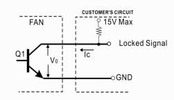
\*Transistor Q1 at "ON" position Collector current.....I<sub>c</sub>=10mA Max Saturation Voltage.....V<sub>oL</sub>=1.0V Max (Between Collector and Emitter at  $I_c$ =10mA) \*Transistor Q1 at "OFF" position Release Voltage.....V<sub>ort</sub>=15V Max
