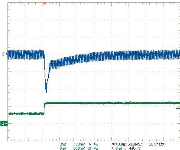
Step Load Transient Response (Vin=12V, Vout=3.3V, Cload=0, Iout=1.5A to 3A) Trace 2=Vout, 100 mV/div. Trace 4=Iout, 2.5A/div.
