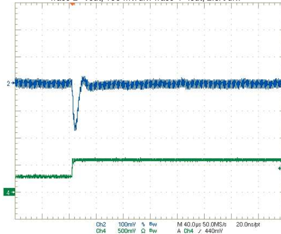
Step Load Transient Response (Vin=12V, Vout=1.8V, Cload=0, Iout=3A to 1.5A)
