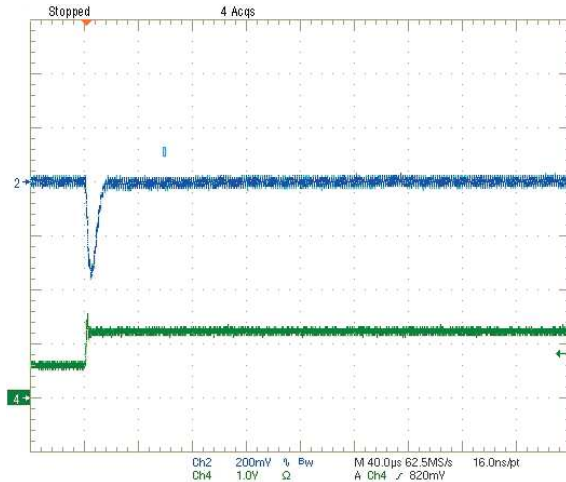
Step Load Transient Response (Vin=12V, Vout=2.5V, Load=0, Iout=3A to 6A) Trace 2=Vout, 200 mV/div. Trace 4=Iout, 5A/div.
