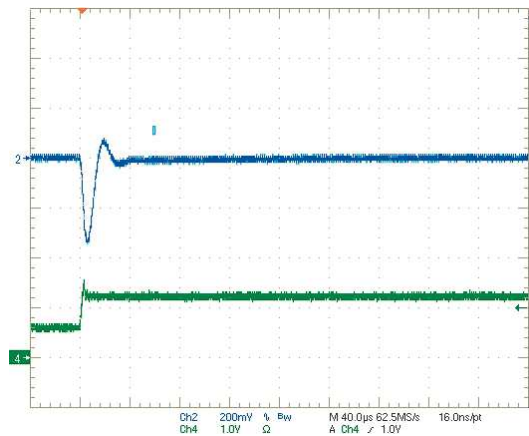
Step Load Transient Response (V in =5V, V out =1.5V, I out =3A to 6A) Trace 2=V out , 200 mV/div. Trace 4=I out , 5A/div.
