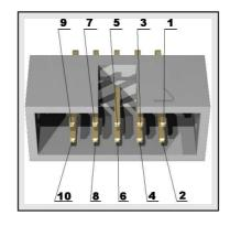
IMPORTANT: Be careful with the voltage levels of the signals of the UEXT and specifically the output available at pin #1. The on-board 3.3V/5V switch also controls the voltage output of the UEXT! Do not connect Olimex modules when the switch is set to 5V position, unless you are 100% sure that these UEXT modules work fine at 5V (most Olimex modules can not work properly at 5V, only at 3.3V)
