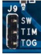
Fig 2. Selection of operating mode using jumper J9
