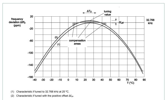
Fig 10. Temperature averaged over application range 5 °C to 45 °C
