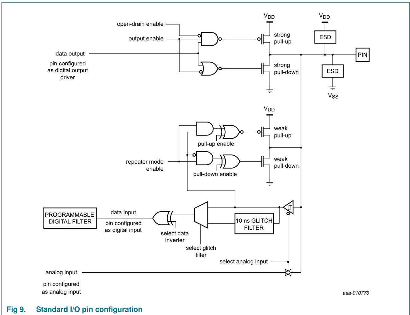
Fig 9. Standard I/O pin configuration
