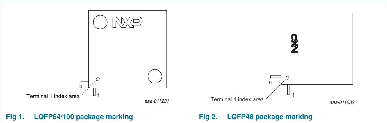
**Fig 1. LQFP64/100 package marking**
