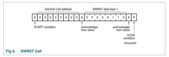
The I<sup>2</sup>C-bus master must interpret a non-acknowledge from the PCA9952/55 (at any time) as a 'SWRST Call Abort'. The PCA9952/55 does not initiate a reset of its registers. This happens only when the format of the SWRST Call sequence is not correct.
