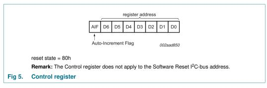
When the Auto-Increment Flag is set (AIF = logic 1), the seven low-order bits of the Control register are automatically incremented after a read or write. This allows the user to program the registers sequentially. Four different types of Auto-Increment are possible, depending on AI1 and AI0 values of MODE1 register.
