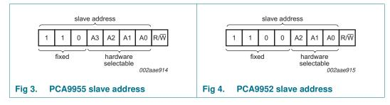
The last bit of the address byte defines the operation to be performed. When set to logic 1 a read is selected, while a logic 0 selects a write operation.
