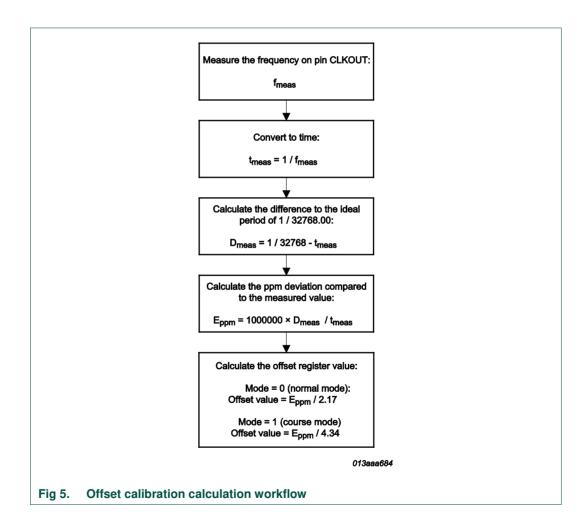
The 32 kHz quartzes are of the tuning fork type and feature a parabolic frequency response over temperature. When the application is dominantly used over a limited temperature range, it is often helpful to tune the frequency to be slightly higher at the
