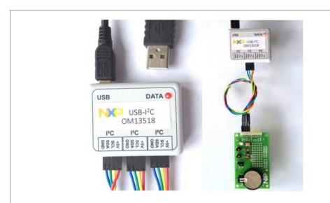
Fig 5. A) Dongle OM13518, B) connected to an evaluation board
